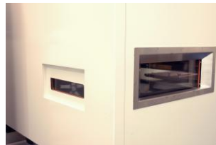
Furnace observation window
